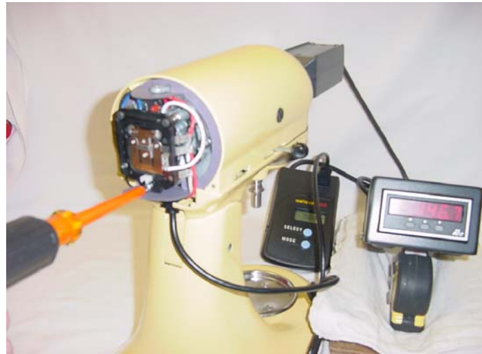
Fig. 79 Adjusting screw at the bottom of the control plate for speed # 6.
