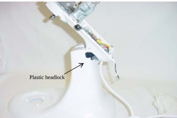
Fig. 74 A plastic headlock has been riveted to the pedestal of international export models. An international model is shown locked in the “inclined” position. This is obtained by the action of the spring loaded lock lever used on these models.
