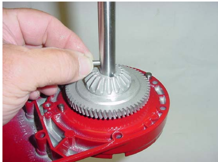
Fig. 53 Remove pin after pushing vertical center shaft up.
