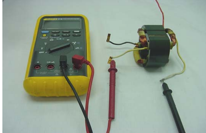
Fig. 35 Test the two stator coils with an ohmmeter set on low scale.
